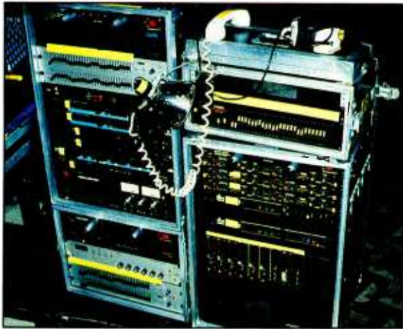
Figure 6. Sun Sound's house electronics racks included Klark-Teknik and Yamaha graphic equalizers, dbx noise gates and compressor/limiters, and various delays and digital reverbs.
