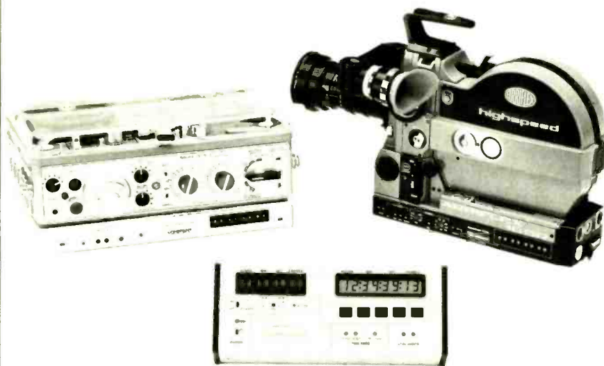
Figure 7. Coherent Communications time code system, including Nagra time code generator, 16mm camera module and master clock.
