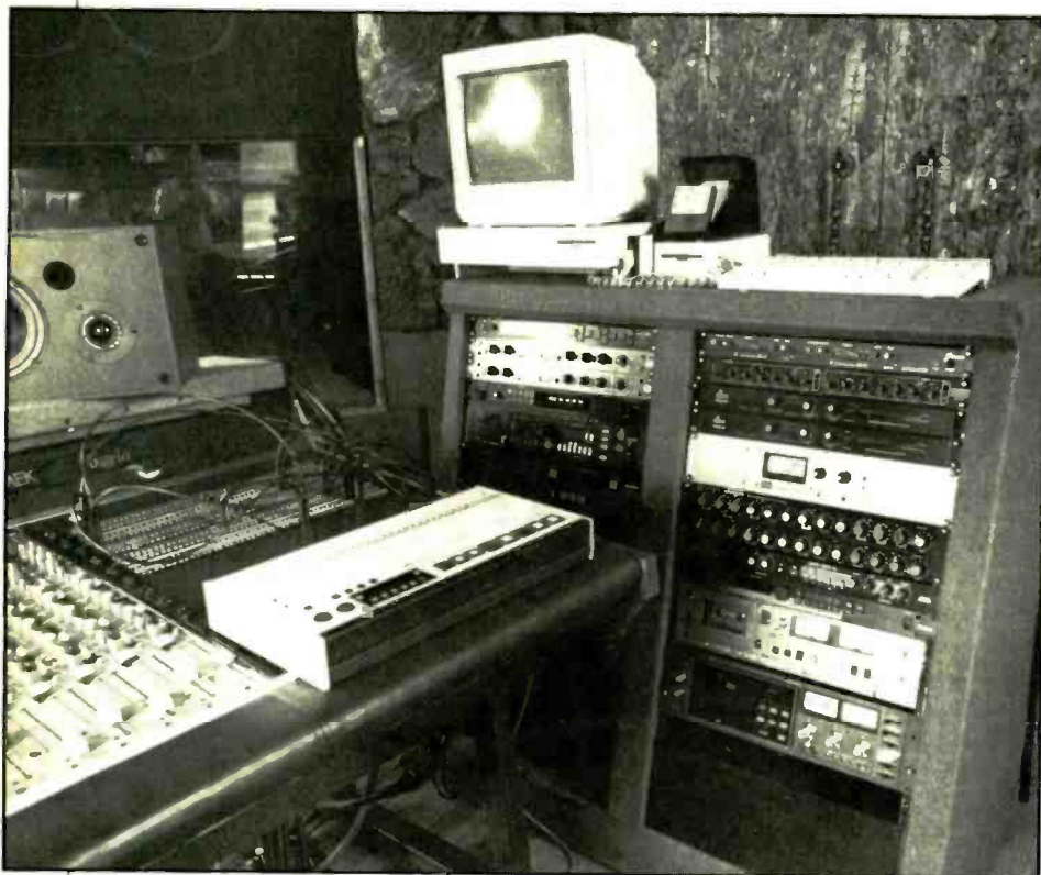
To the left of the 36-input Amek Angela console are a pair of movable equipment racks that house a wide selection of signal processors. Located on top of the rack is an Amiga PC plus companion MIDI sequencing and music librarian software.
