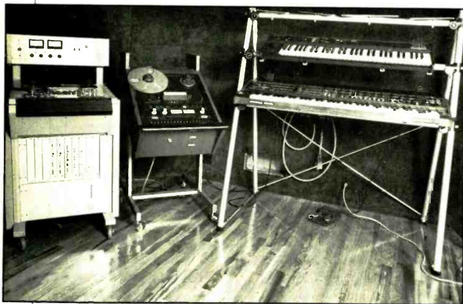
Across the control room, a second equipment soffit houses an Otari MTR-12 mastering deck, an Otari MX-5050 2-track and an Ultimate Support rack housing an Oberheim Xk and a Sequential Circuits Prophet T8.
