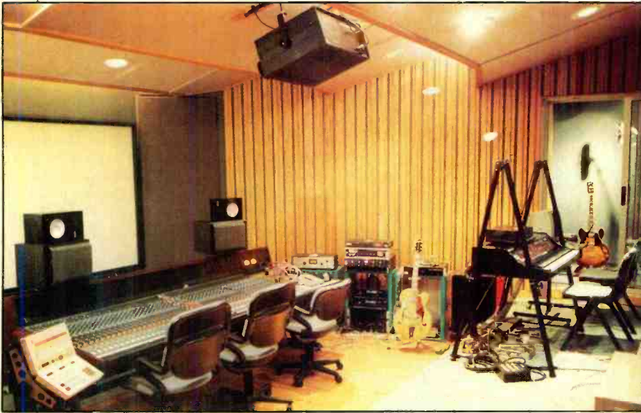
Studio C's 3-tiered control room features a 60-input customized Amek model 2500 console with Audio Kinetics MasterMix automation, a custom Keith Klawitter monitoring system, Electro-Voice Sentry and Yamaha NS-10M close-field monitors, an Otari MTR-90 24-track, an overhead video projection system and screen, plus various synthesizers and effects. To the right can be seen the entrance to a dedicated vocal and instrumental overdub booth.
