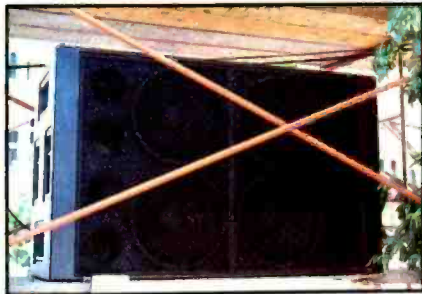
Figure 10: Subwoofers supplied by Stage Audio comprised EAW SB550L enclosures, each housing four RCF L15/P200 drivers.
