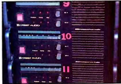
Figure 11: Stage Audio uses Crest Model 3000 power amplifiers to drive midrange and high-frequency components.
