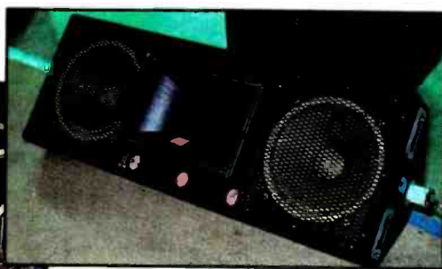
Figure 6: Custom floor slant monitor speaker enclosure developed by M.D. Systems for Steppenwolf.
