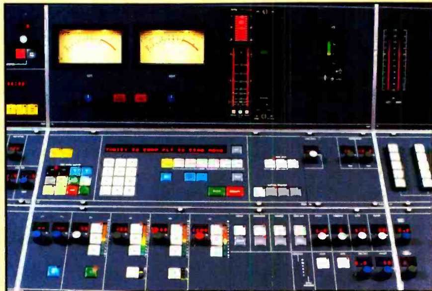
Closeup of the DSP disc-mastering console in Disc 1, which enables all front-panel settings to be stored and recalled for subsequent recuts from digital master tapes.
