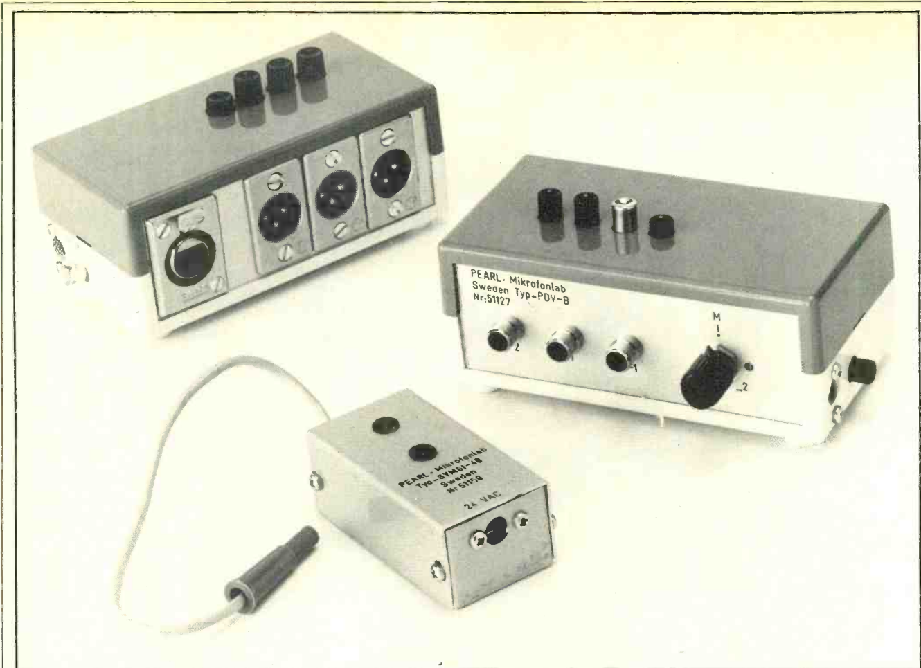
Accessories include the PDV-B switcher unit, which provides various mono/stereo output combinations (shown top left and right), and the SYMSI-48 power supply module.
