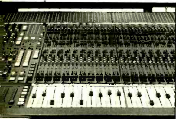
Overview of 48-input custom Cherokee console. At left is the master control section.
