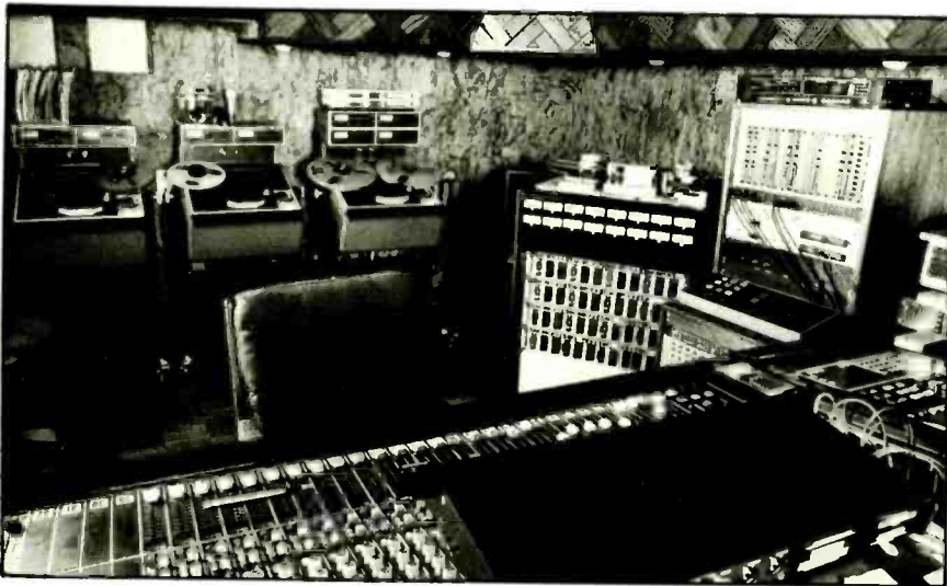
Crest Video's audio-for-video mastering room uses Ampex ATR-102 2-track and -104 4-track, plus an MM 1200 16-track (shown here with 1-inch 8-track head blocks). The room's outboard equipment includes (from top right) an Eventide Harmonizer, Audio+Design Scamp Rack, Dolby 360 units (for use with an outboard CAT. 43 Cinema Processor), Quantec Room Simulator, control panel for an EECO MQS-100 timecode synchronizer, plus custom designed remotes for multitrack and mastering machines.
