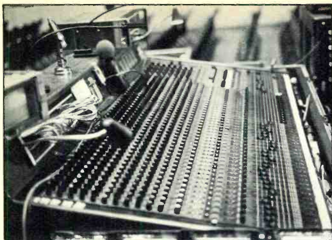
Figure 2: (Shown left) Jim Gamble Associates' HC-40-24 mixing console as supplied to the Grateful Dead by Ultra Sound. Figure 3: (Shown right) Ultra Sound packages its Crest amplifiers in two different types of racks. Four Model 4000 units are housed in compact racks, while larger systems use five Model 3500 and two Model 5000 amplifiers per rack.
