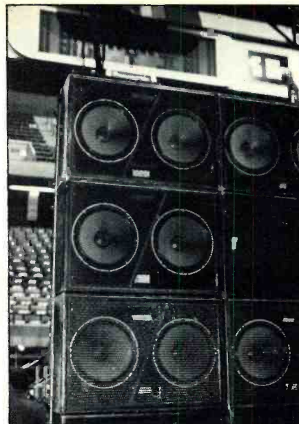
Figure 7: 650-R2 subwoofers were stacked five high in rows of three, for a total of 30 boxes in use at the Meadowlands performance.
