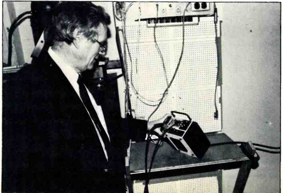
Engineer Bill Busiek with a video transmitter unit at Symphony Hall used for relaying digital audio encoded with a dbx Model 700 CDPM processor back to the WGBH studio.
