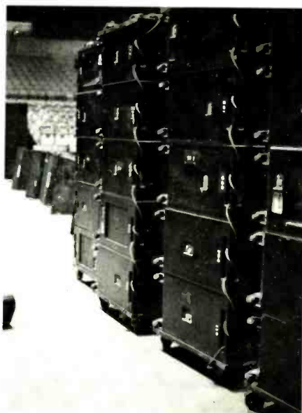
Figure 4: The stacked boxes are secured with steel safety cables. Nylon ratchet straps around the edges hold the five boxes and metal frames together in a cohesive unit.
