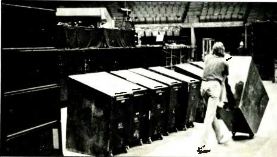
Figure 3: Two permanent wheels and an integral handle offer ease of transport of the trapezoidal boxes by one stage hand.
