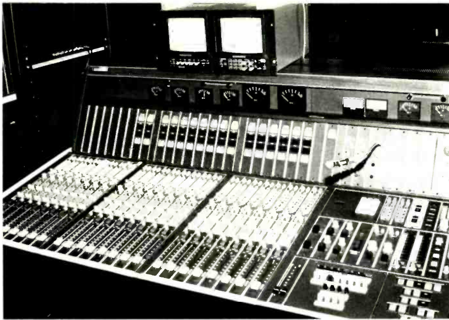
Studio 64, the Audio Integration Room at ABC Los Angeles, features a stereo McCurdy production console. This area, which also serves to back up the facility's main network commercial break studio, is used to route audio to air during sports remotes, and to provide network commercials that are added along with regional rollovers.
