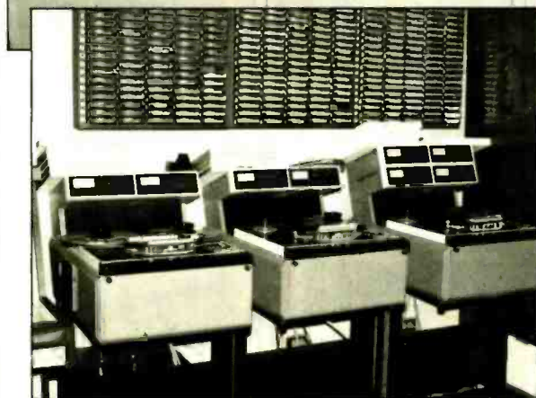
Video Sweetening and Remix Studio C features computer control of SMPTE synchronization and cueing (above) plus a full effects library on NAB cartridge (left).
