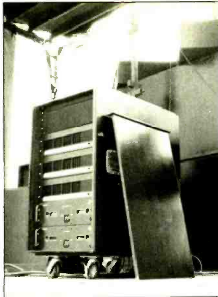
Figure 11: Amplifier racks house two QSC Model 1400s, and three 1200s; Model 3800s are provided for low frequencies.
