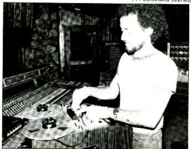
... Engineer Steve Toby (Fantasy Studios) performing a manual edit on the Mitsubishi X-80 Digital Recorder
