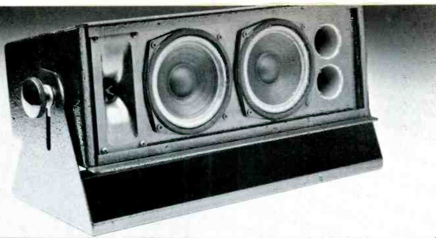
Front view of UPM-1 "quasi" three-way cabinets utilized for delay speakers at 15 locations within the audience seating area.
