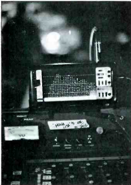
Figure 10: An Ivie IE-30A real-time analyzer, mounted at the monitor console position, offers a third-octave readout of program material.
