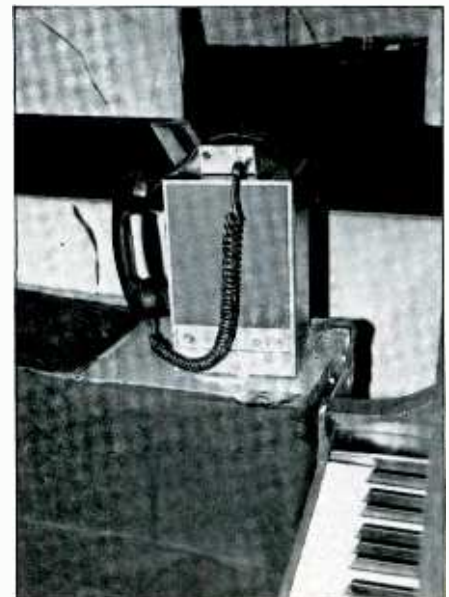
Figure 7: A Yamaha MS-10 self-powered mini-monitor offers a reinforced piano signal to the conductor.
