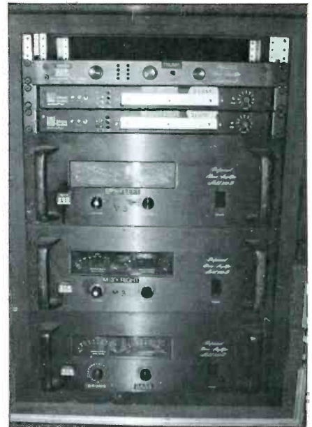
Figure 11: Meyer M-1 and M-3 processors and BGW 750W stereo power amplifiers drive various Meyer on-stage loudspeaker monitor cabinets.
