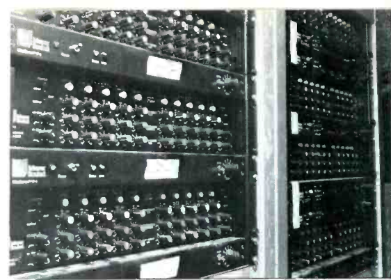
An equipment rack houses the P-1 processors for the UPM-1 delay speakers, and CP-10 complimentary phase equalizers
