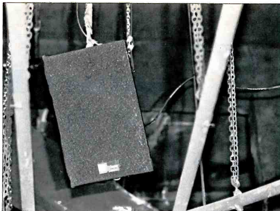
Sidefill monitors comprised a pair of Meyer UPA-1A two-way cabinets suspended above either side of the stage area from the catwalk.
