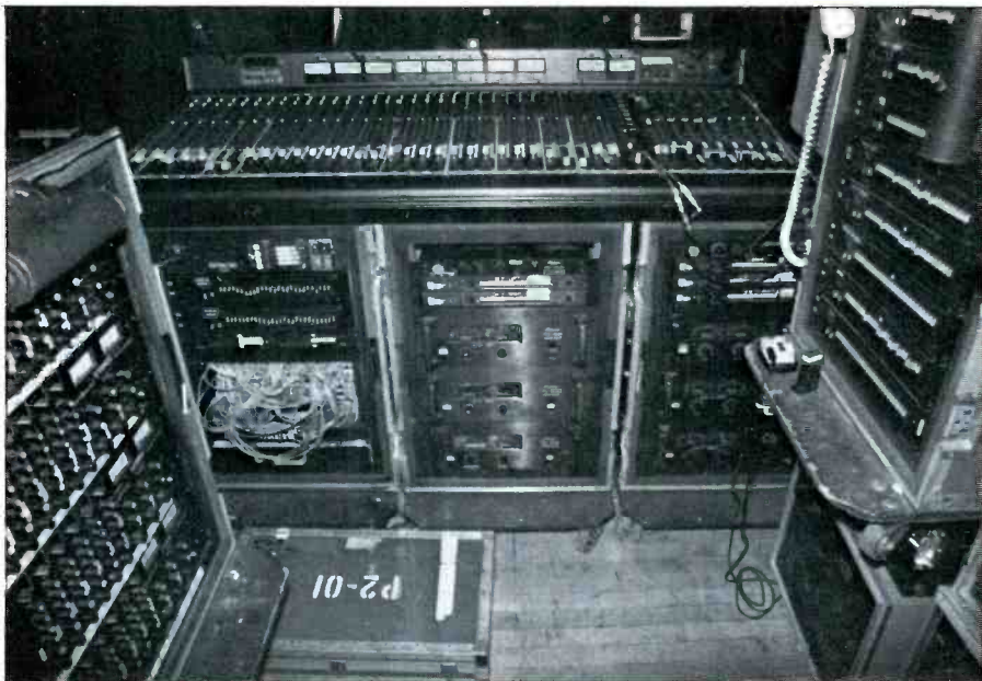
Figure 8: The monitor position (stage left). A Soundcraft 800B console forms the heart of the on-stage monitoring system.
