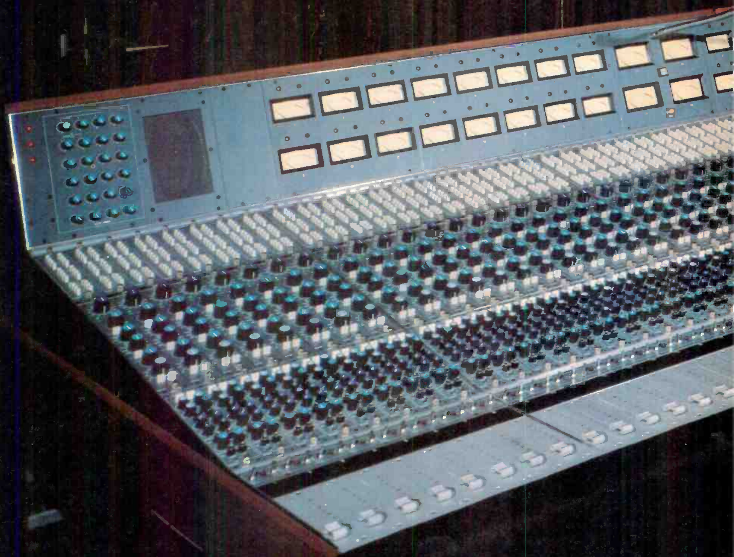
Picture shows one of three studios at Motown Recording Studios—Los Angeles equipped with the ultimate 8078 console and the NECAM Computer Assisted Mixing.
