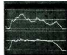
Frequency response of the speaker and room in a monitor system. The top trace, with 40dB window between reference lines, is before equalization, the bottom trace after equalization. The source was pink noise and the plots were made using the spectrum analysis mode with a 1/2-octave bandwidth.
