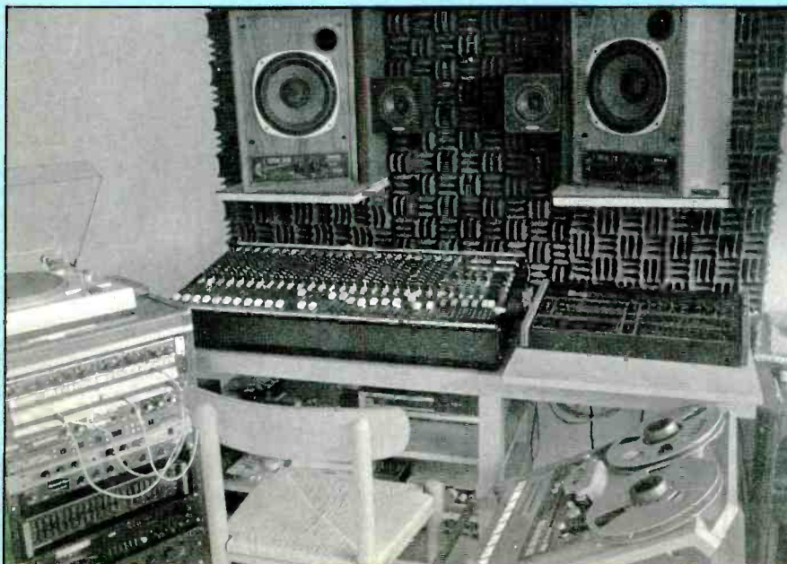
Monitors form a 1 meter equilateral triangle with the engineer's head. Equipment rolls into a convenient position for recording.
