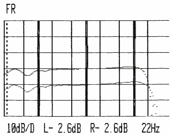
Fig. 1: Otari MX-5050-MKIII-8: Frequency Response Plots at 15 ips (A) and 7½ ips (B) using Scotch 226 tape. Cursor is set to show approximately -2 dB low frequency cut-off point.
