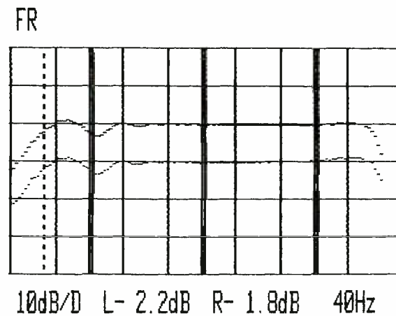
Fig. 1: Otari MX-5050-MKIII-8: Frequency Response Plots at 15 ips (A) and 7½ ips (B) using Scotch 226 tape. Cursor is set to show approximately -2 dB low frequency cut-off point.
