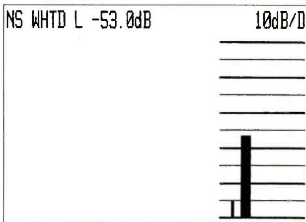
Fig. 6: Akai GX-625: Signal-to-noise ratio at 3¼ ips, re: 0 dB record level.
