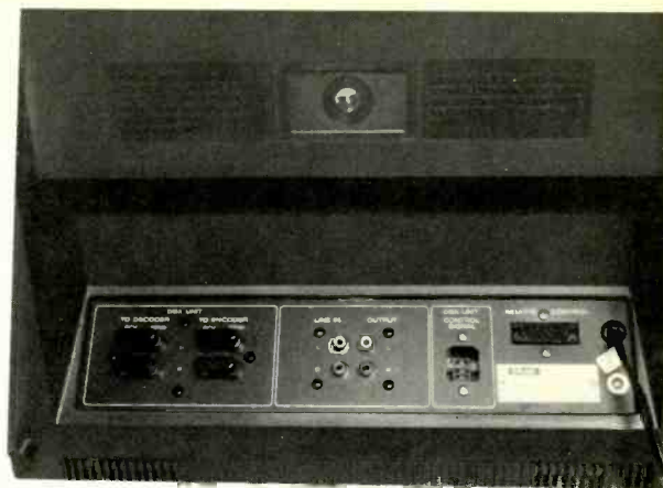
Teac X-10R: Input and output line terminals at rear are sloped for easy access.
