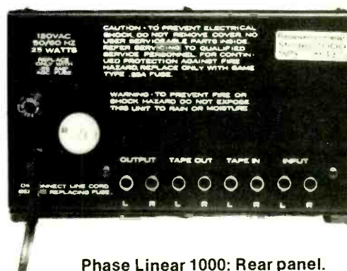
Phase Linear 1000: Rear panel.
