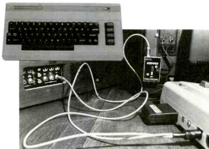
A DIN ADAPTER lets you route the 64's audio and composite video outputs separately, as above. A built-in RF modulator allows direct connection to a TV set.
