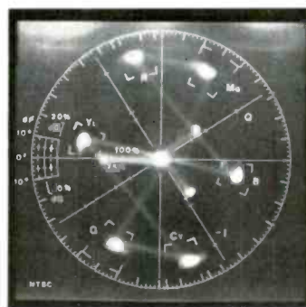
VCR COLOR ACCURACY in Beta II (left) and Beta III (right). The fuzziness of the color vectors (the white dots in the six target squares) is caused by chroma noise. Even so, the SL-2700's superb performance is clearly evident, bettering that of any TV tuner we have yet tested. Chroma level (color saturation) is indicated by a dot's radial distance from the center of its target, while chroma phase (hue) accuracy is indicated by its angular displacement. Both are just about right on the money, in Beta III as well as Beta II.
