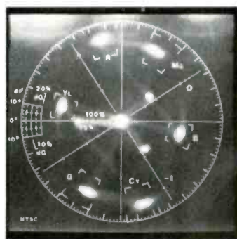
VCR COLOR ACCURACY in Beta II (left) and Beta III (right). The fuzziness of the color vectors (the white dots in the six target squares) is caused by chroma noise. Even so, the SL-2700's superb performance is clearly evident, bettering that of any TV tuner we have yet tested. Chroma level (color saturation) is indicated by a dot's radial distance from the center of its target, while chroma phase (hue) accuracy is indicated by its angular displacement. Both are just about right on the money, in Beta III as well as Beta II.
