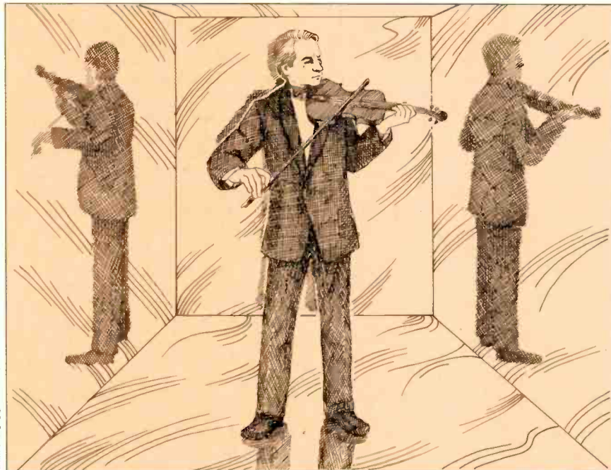
Fig. 2. Acoustically, a concert hall is a large room constructed with acoustical mirrors: the walls, floors, and ceiling. Each mirror image shown here represents a principal sound reflection.
