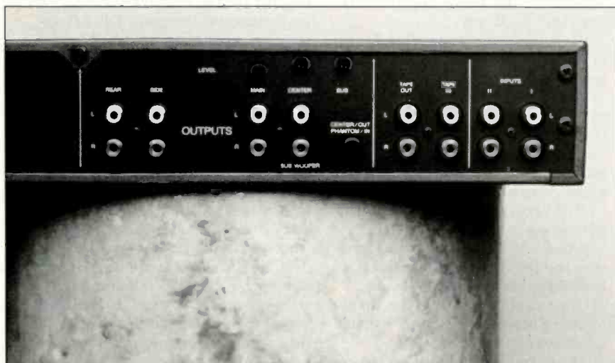
The back panel of the CP-1 contains dedicated center-channel and subwoofer outputs, plus a phantom-center switch for systems without a separate center speaker. Level-trim controls are provided for all outputs, as are connections for a tape deck (which can be switched to record processed signals).
