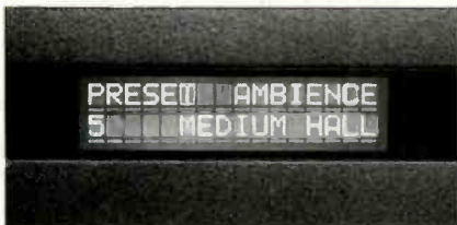
The CP-1's liquid-crystal display shows all operating modes and settings.
