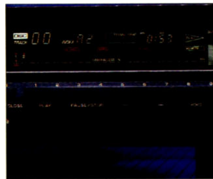
On the right is the column indicating the digital volume-control setting of the CDX-1100U.
