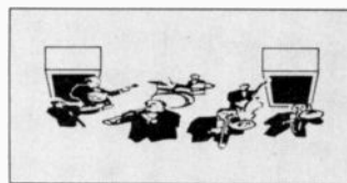
Conventional stereo: The sound is heard, more or less, on a flat curtain of sound between the two speakers. Volume differences only. The timing cues are gone.
