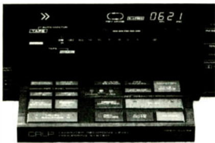
THE GX-R99'S RECORDING CONTROLS (INCLUDING CRLP) ARE IN A MOTORIZED DRAWER.
