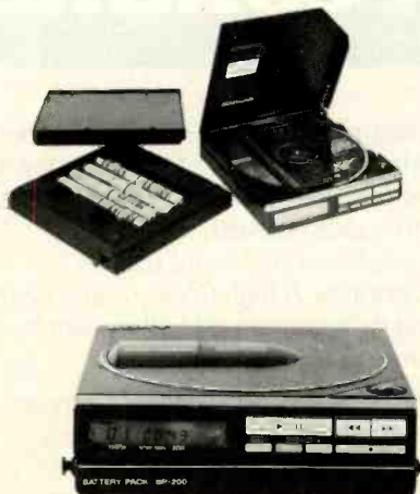
New circuits led to more compact design of Sony's D-7 Discman CD player, which includes battery pack.
