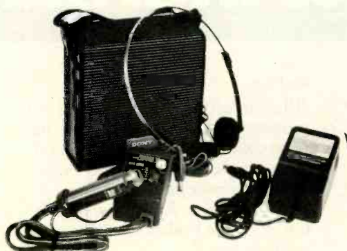
New circuits led to more compact design of Sony's D-7 Discman CD player, which includes battery pack.
