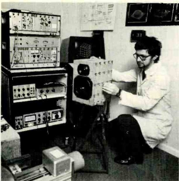
Manufacture and design at B&W: Worker assembles mid-range/tweeter heads for 801F and 802F speakers (top); interferometry setup (middle left), with laser at right and the driver under test in jig at left; automated woofer test station (middle right); r&d engineer Glyn Adams investigates cabinet vibration modes in laser lab.
