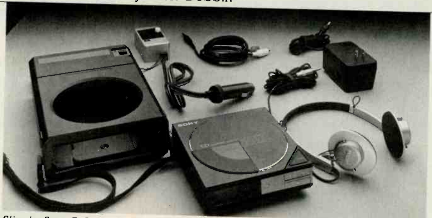
Slip the Sony D-5 into its carrying case/battery holder (left), and you have a personal-portable CD player. Adapters (rear) enable it to be used at home and in the car.
