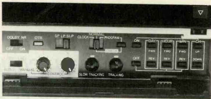
SECONDARY CONTROLS are behind a flip-down door at the bottom of the front panel. They include an ALC (automatic level control) switch, manual recording-level controls, tracking adjustments, Dolby B and recording-speed switches, an OTR (one-touch recording) button, and, to the right, the timer programming controls.
