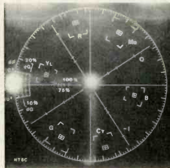
COLOR CONSISTENCY of the PV-1730's recorder section (left) and for its TV tuner (right). In each case, the ideal would be for the cluster of dots toward the left edge of the grid to be a single dot at the intersection of the nine-o'clock axis with the circumference. The radial spread of the dots indicates chroma differential gain—a measure of how much chroma level (color saturation) varies with changes in scene brightness (luminance). The angular spread shows the chroma differential phase, which tells how much chroma phase (hue) shifts with changes in brightness. The VCR's performance is, again, perfect, and the tuner's is excellent, with nearly all of the error concentrated at the highest brightness level.
