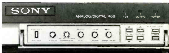
THE KX-1901A'S CONTROLS are behind a flip-down panel. As long as the master power switch at the far left is on, the monitor remembers its last PICTURE, VOLUME, and RGB/NTSC settings even when it has been turned off with the regular power switch. Three lights above the right end of the control panel indicate system status.
