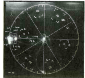
TUNER COLOR CONSISTENCY is excellent: Chroma differential phase and gain are both very low. Differential gain (how much color saturation varies with scene brightness) is indicated by the radial spread of the color vectors (dots). Differential phase (how much hue varies with brightness) is shown by their angular spread.
