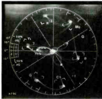
4-degree clockwise phase rotation to simulate the best color one could obtain using the tint control on a monitor. This puts all six color vectors (represented by white dots) on target.
