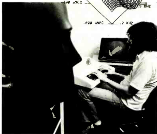
A DUMMY HEAD with microphones in its ear canal helps researchers at AR determine the imaging characteristics of a pair of loudspeakers. The head "listens" to sounds and then feeds data to a computer equipped with a model of the human auditory system. The resulting three-dimensional plots depict the difference in arrival time at the two ears at various frequencies.
