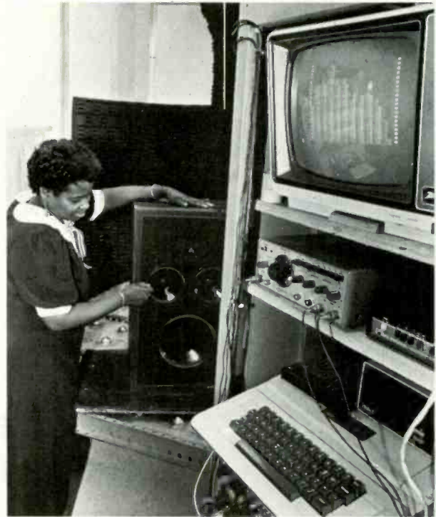
FINALLY, MOLLY JONES , a quality-control technician, evaluates finished systems with an Apple-based program that performs impulse-response analysis, one-third-octave frequency response measurements, and driver-phasing and system-impedance checks.
