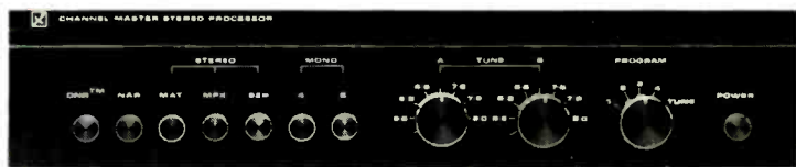
PICKING UP SATELLITE stereo broadcasts often involves tuning in two subcarriers. Meters on the KLM (top) and presets on the Channel Master simplify the process.
