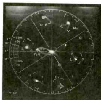
TUNER COLOR ACCURACY is good. The vectorscope photo at left indicates low color saturation (chroma level) and a small amount of hue (chroma-phase) inaccuracy. The photo at right—made with 4 1/4 dB additional chroma gain and approximately 7 degrees of clockwise phase rotation—simulates the best results one could obtain using the color and tint controls on a monitor. With this adjustment, performance is excellent.
