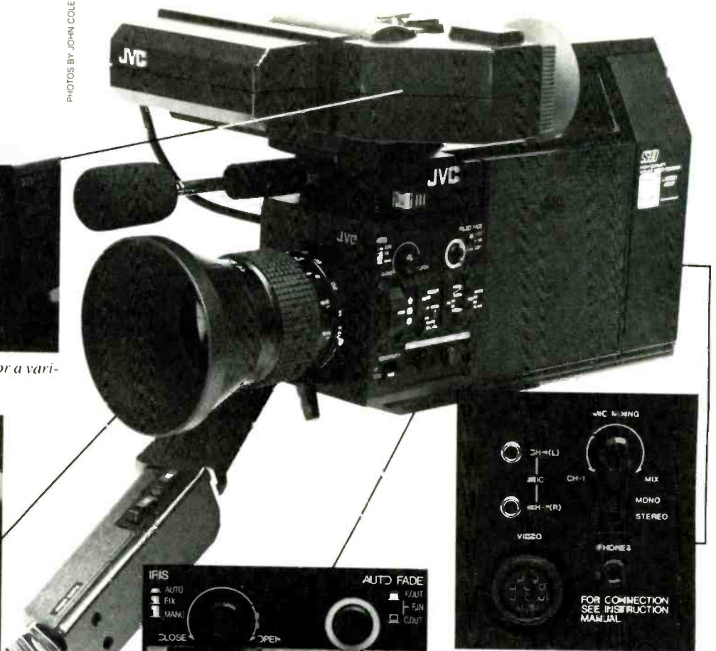
A panel on the camera's aft end contains VCR connector, mike inputs, audio mixing controls, and headphone output.
