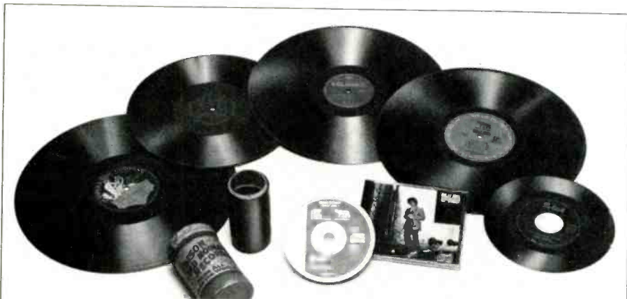
The Compact Disc (foreground, center) and its forebears (clockwise, from left): the Edison wax cylinder, acoustical and electrical 78s, and 33- and 45-rpm microgroove discs
