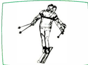
Incompatibility of head-gap slant with that of signal recorded by opposite head produces jumpy, blurred picture
