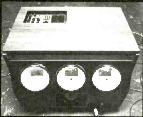
The console of the NovaBeam two-piece projection system contains the basic video chassis and tuner as well as three separate Novatron tubes.
