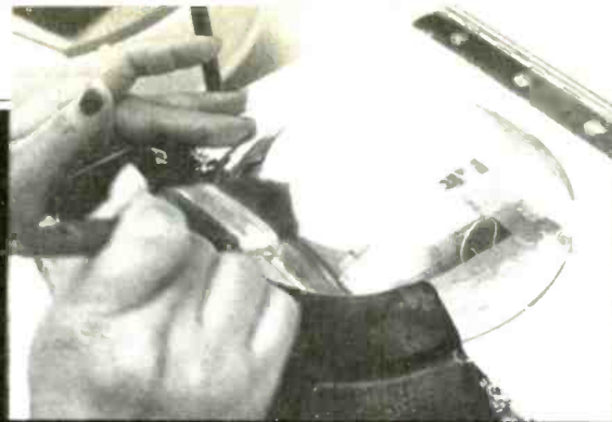
A worker in the Kloss Video Corporation factory applies the phosphor coating to the spherical surface of the Novatron faceplate. The faceplate also serves as part of the vacuum system and lens arrangement.
