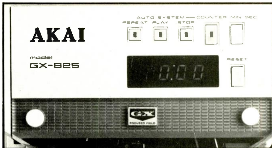
The display on the GX-625 is switchable to counter or timer modes. With the counter, the REPEAT, PLAY, and STOP keys allow for cassette-deck style automation.
