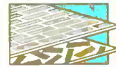
The pure chromium dioxide particles in the PRO II, unlike ferric oxide particles, are homogeneously shaped and uniformly sized to give that tape superior performance
