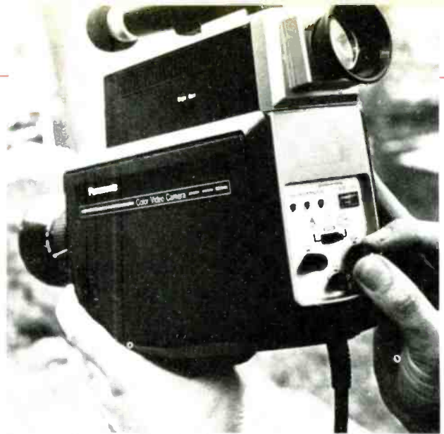
Author adjusts the blue color balance on the Panasonic PK-600 camera, then (next page) sights and shoots.
