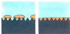
Discwasher D3 ® solution (left) beads up on the grooves. Sound Life (right) with super-wetting action deep-cleans grooves.
