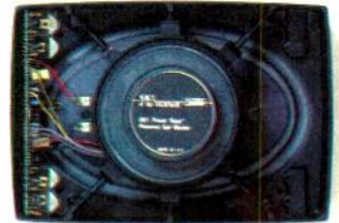
Rear view of the Power Bass, showing built-in amplifier. When added to any tape player or radio, the Subwoofer bi-amplifies the system, improving the dynamic range and reducing distortion.
