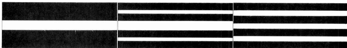
Original mono cassette layout (left) was adapted to four-track stereo (center) for interchangeability; equal guard bands to minimize crosstalk in multichannel use (right, for Teac 144) compromise compatibility and sound. See text.
