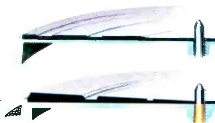
The ordinary platter mat is flat. Ours is concave to compensate for warped records.
