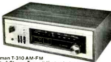
Luxman T-310 AM-FM Dolby Stereo Tuner IHF sensitivity 1.7 uv. Selectivity 75dB. Capture ratio †5dB. Total harmonic distortion: 0.1% @ 400 Hz, mono; 0.12% @ 400 Hz, stereo. Dolby B-type circuits for decoding FM and tapes. Dolby calibration controls. Switchable/variable AM/FM muting. Dimensions: 19 1/8" x 11 1/8" x 6 1/2". Weight: 21 lbs. $595.00
