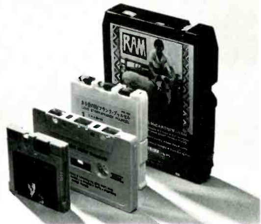
From the left these are the Faraday Cartrette, a cassette, the Hipac cartridge, and a stereo-8 cartridge. Head openings are in narrow edge of all but Cartrette.
