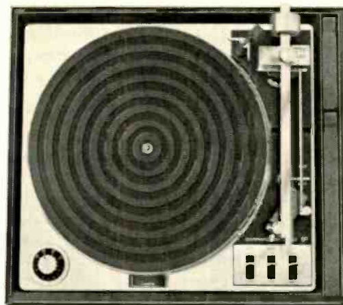
Articulated arm on Garrard Zero-100 adjusts offset angle of head, keeping stylus tangent to groove.
