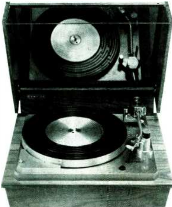
Empire's latest, the Troubador model 598, bears a resemblance to earlier models but has been redesigned so that it can be used at extremely low tracking forces.
