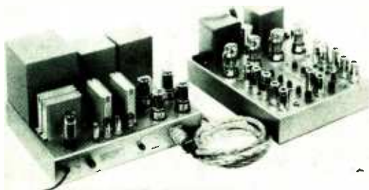
Dual 100 power amp; amplifying channels and power supply occupy separate chassis.
