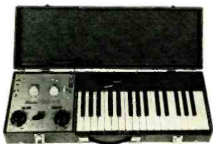
Allen's "Flying Hammers" (above) consist of a row of weighted metal springs, one for each key, that begin bobbing when a key is struck. Keys run out of picture to right; springs are in center. As they bob, they make and break contacts at left, producing a "repeat tone." Some typically all-electronic instruments are shown at left (melody instrument) and below (rhythm section).
