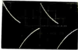
Square-wave response to 50 Hz.
