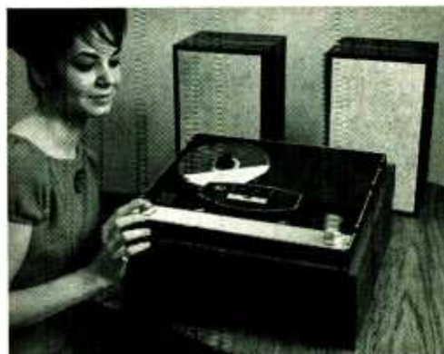
Ampex 1450 deck features automatic reverse for play-back and self-threading take-up reel under cover.
