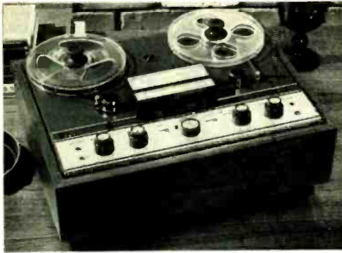
Magnecord 1020 two-speed deck is available factory-built or in kit form from Heath Co. as Model AD-16.
