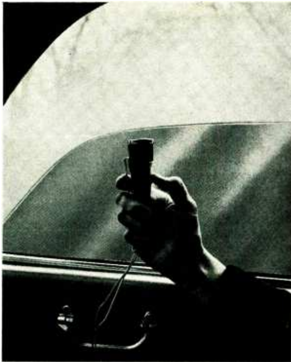
Partly closed car window shields mike from wind while permitting wanted sounds to be captured.
