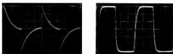
Square-wave response to 50 Hz, left, and to 10 kHz.
