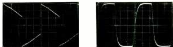
Square-wave response to 50 Hz, left, and to 10 kHz.
