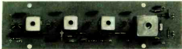
IF strip in Scott receiver before and after integrated circuits. Simplified strip actually boasts more parts.
