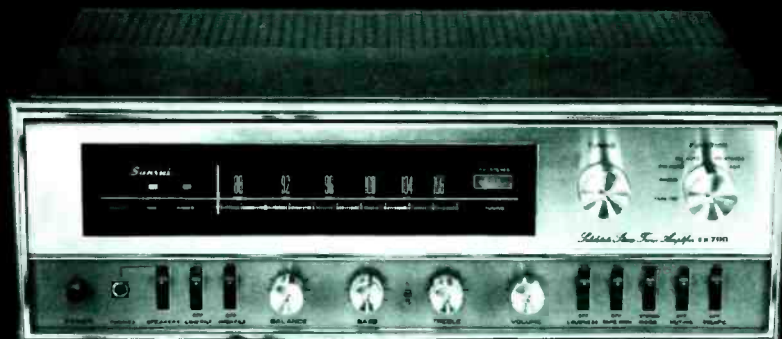
Model TR-700—Solid State Multiplex Stereo. Music Power: 60 Watts @ \pm 1 dB. FM Usable Sensitivity: 1.8\mu\text{V} \pm 3 dB (IHF).
