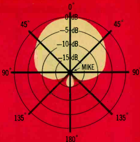
UNI-DIRECTIONAL One side of diaphragm is partially exposed to air; other side fully exposed.
