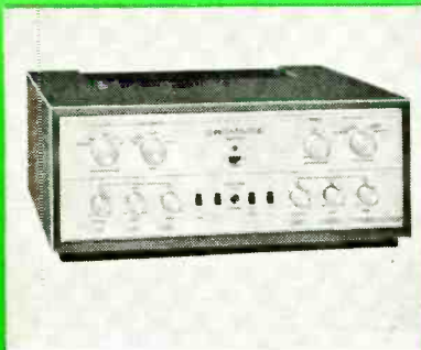
Md. 3000 Grommes President Line 100% solid state stereo preamp/amplifier. 120-watt, 60-watt per channel. Freq. Response: 20-20,000 cps at 50-watt; Distortion: Harmonic- 0.3% at 1000 cps, Intermodulation- 0.5% at 50-watt. $299.95. Grommes-Precision, Franklin Park, Ill. (45)
