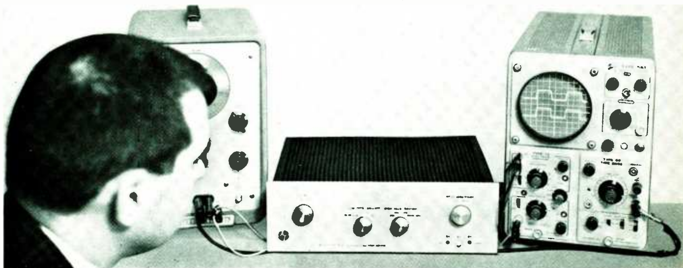
A fascinated audiophile at the 1962 New York hifi show observes the remarkable square wave response of the Acoustech I (the bottom pattern is the 20 KC output of the square wave generator . . . the top wave is the output from the Acoustech I).
